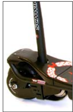
Drive train on the 300, 4.0 and 400 series scooters
