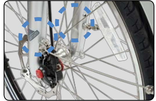
Fender standoffs, bolted to fork
