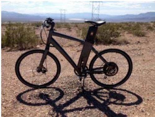
Driving this bike is a strong, silent and sophisticated 500 watt gearless hub motor. It's capable of moving larger riders, scaling moderate hills and it even offers regenerative braking to extend range. I'm a big fan of gearless hubs and appreciate the fact that eFlow integrated regenerative braking because it saves your brake pads! The truth is, it doesn't offer a lot of actual "regeneration" but if you have a long hill, it's nice to recoup some while reducing the heat and wear on your discs.
