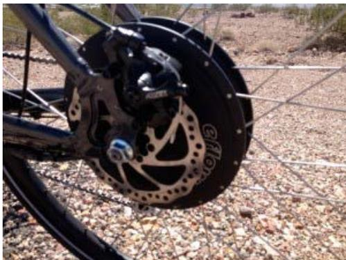
Speaking of stopping power, this bike has disc brakes front and rear, though not hydraulic. The overall weight of ~50lbs (depending on frame size) is decent but not as light as I would have liked for a road style city bike. I do like the fact that they offer three frame sizes in the high-step and two in the low-step because it means you can actually enjoy riding this bike vs.
